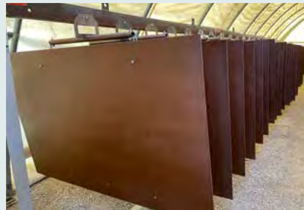
Weathering steel has become so popular that California Sheet Metal has a structure on its property dedicated to giving the metal its aged look.
